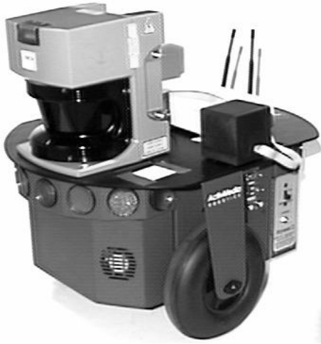
Figure 1: Player can control many popular robot devices, including the Pioneer 2-DX mobile robot and peripherals pictured here.
