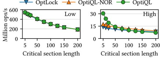
**Figure 8:** Lock throughput under varying critical section lengths (80 threads). Opportunistic read mainly benefits short reads.
