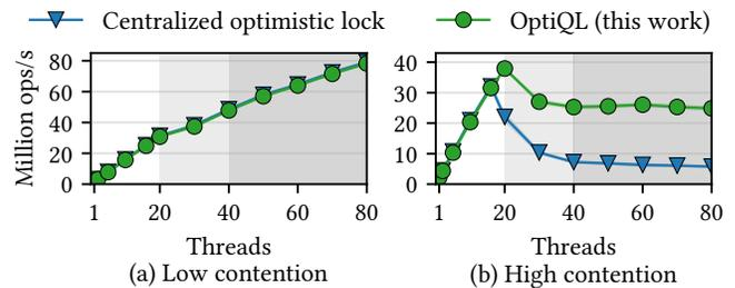
**Figure 1:** Update throughput of a memory-optimized B+-tree on a 80-thread server. Centralized optimistic locks work well under low contention (a) but can collapse under high contention (b). OptiQL performs well in both cases.
