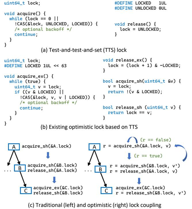
**Figure 2:** Existing optimistic locks extend spinlocks (a) to support optimistic readers (b). The similar interfaces allow easy adaption in lock coupling protocols (c).
