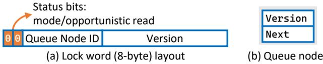
**Figure 3:** OptiQL structures. (a) The lock is still 8-byte but carries more information. (b) A queue node (for writers only) includes a version number and a pointer to the next writer.
