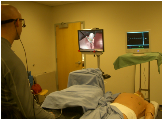
Figure 2: Experimental setup with display monitors, training dummy, and head-mounted eyetracker
