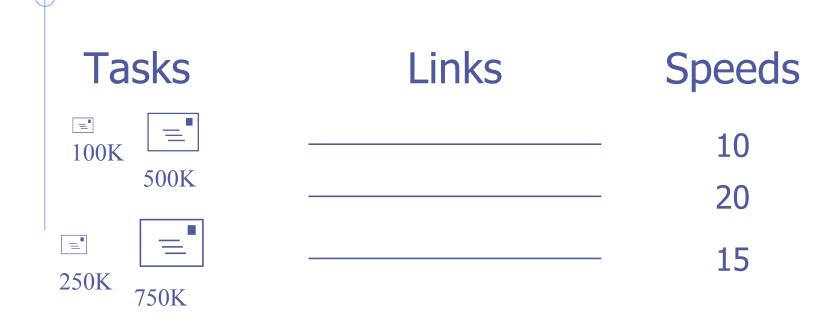
delay of task w on link l = w / (speed of l)
