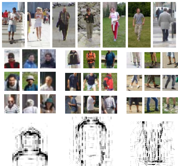
Figure 1. First row shows examples of pedestrian images. The next three rows show three local regions within the pedestrian windows. The last row shows the shapelet features learned by our algorithm for each of the three regions.
