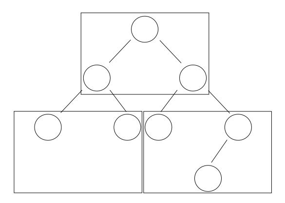
Nodes of a binary tree can be located in different blocks on a disk.
