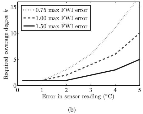
FIGURE 27 The tradeoff between the accuracy in sensor reading and the required coverage degree, given a maximum tolerable error in the FWI index. (a) considers a wide range for sensor accuracy, while (b) zooms in the small range between 0–5.
