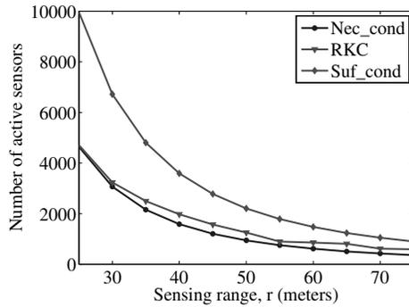
FIGURE 17 Efficiency of our centralized  $k$ -coverage algorithm (RKC). The figure compares the number of active sensors produced by our RKC algorithm versus the necessary (Nec\_cond) and sufficient (Suf\_cond) conditions proved in [34].
