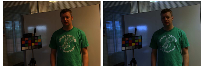
Fig. 2. A scene with two distinct illuminants. The image on the left is colour-corrected using outdoor sky-light and the image on the right is colour-corrected using indoor light.
