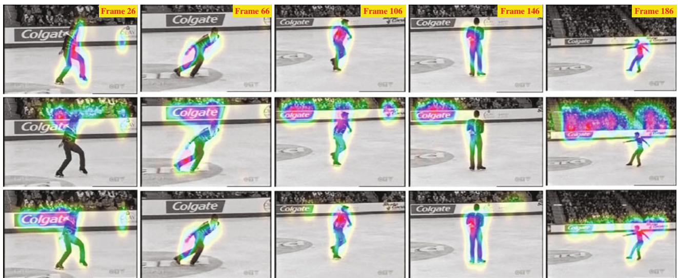
Figure 8 Comparative tracking results for “skate” sequence by our proposed algorithm ( top row ), without cPoB keypoints filtering ( middle row ), and without keypoints classification ( bottom row ).
