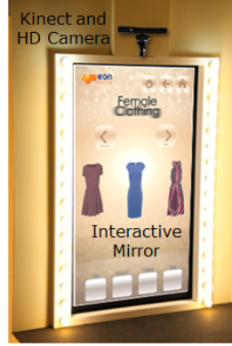
Fig. 1: The front view of the Interactive Mirror with Kinect and HD camera placed on top.
