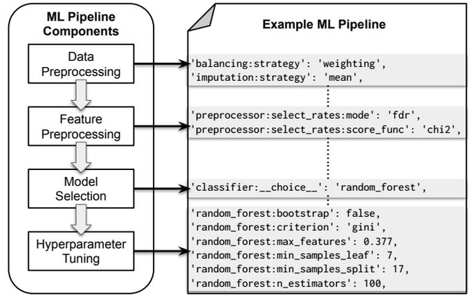
Fig. 5: An example ML pipeline generated by auto-sklearn.
