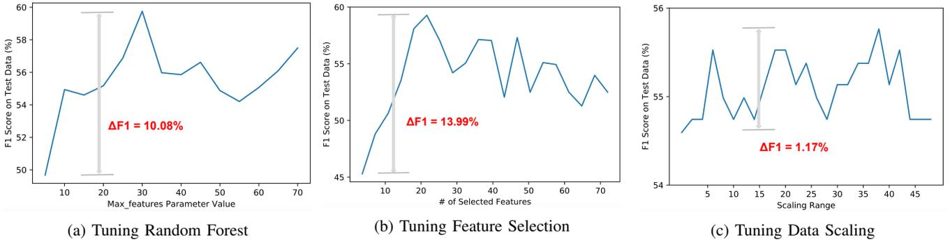
Fig. 3: The effect of tuning parameters for ML pipeline components.
