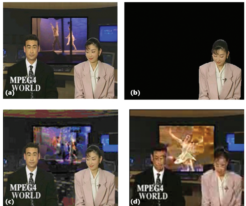
Figure 6. An example of the video object concept and content scalability in MPEG-4. (a) The scene consists of five objects, including two announcers, the caption, ballet stage, and background. (b) One object shown separately. (c) A user indicates that the background and ballet dancers are less interesting, and consequently some packets of these two objects are dropped to meet the bandwidth constraints. Without content scalability, packets are uniformly dropped across the whole rectangular frame, resulting in (d) poorer subjective quality.
