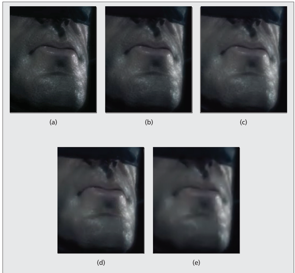
Figure 5. Image quality comparison: a) master image; b) local capture (PSNR:33.85 dB, SSIM:0.97); c) Online: 10 Mb/s connection (PSNR:26.58 dB, SSIM:0.94); d) Online: 6 Mb/s connection (PSNR:26.53 dB, SSIM:0.92); e) Online: 3 Mb/s connection (PSNR: 26.03 dB, SSIM:0.89).
