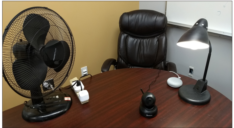
FIGURE 2. Left to right: smart plug, motion sensor, camera, central hub, smart lightbulb.
