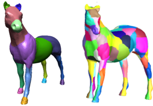
Figure 5: Two different types of mesh segmentation: part-type segmentation (left, taken from [LLS*05]) and surface-type segmentation (right, taken from [SSGH01])
