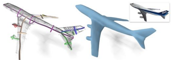
Figure 13: The real airplane object (inset) contains non-cylindrical parts and the input point cloud (left) is incomplete. Yet, our approach successfully reconstructs a 3D model (right) that respects the raw scan and is close to the real object. Different branch paths processed by morfit are shown in different colors.
