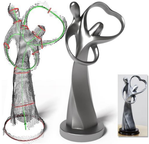
Figure 1: A sparse and incomplete point cloud (on the left) acquired by scanning a shiny metal artwork (in the inset) is interactively reconstructed (in the middle) by our morfit technique with sweeping red profile curves (geometry control) along its green skeleton (topology control).
