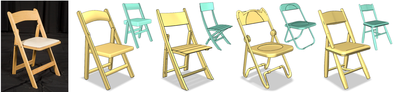
Figure 1: Photo-inspired 3D modeling of a chair from four different 3D candidates (cyan). The new models (yellow) are created as geometric variations of the candidates to fit the target object in the photo while preserving the 3D structure of the candidates.
