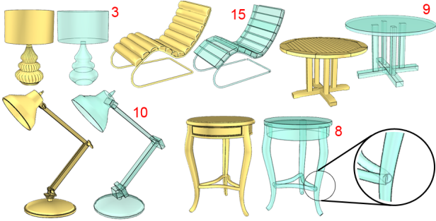
Figure 6: Fitting controllers to 3D models. Cuboids and generalized cylinders allow close approximations of many man-made shapes with relatively small controller counts (numbers in red).
