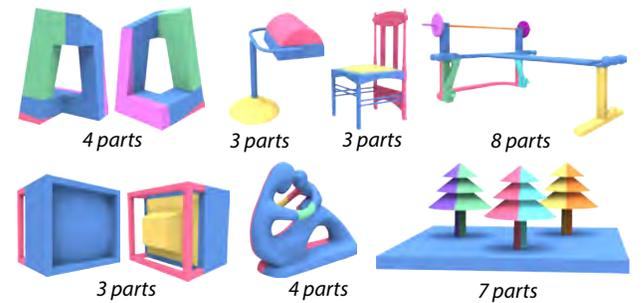
**Figure 16:** Pyramidal decompositions computed by our algorithm which achieve the best material savings (5), in contrast to last two rows of results in Figure 15. Part counts are marked in figure.
