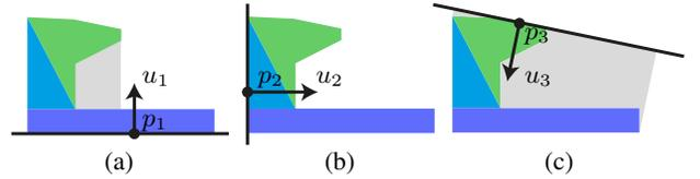
**Figure 11:** Pyramidity estimate. A part combined by three blocks with pyramidity estimated for three up-vectors.  $p_i$  is the one of the lowest points of the part along  $u_i$ . Pyramidal deficit regions are shown as gray areas. Pyramidity score is maximized along  $u_2$ .
