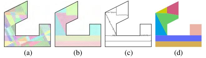
**Figure 8:** Block generation. (a) Cells. (b) Result of cell clustering. (c) Initial block boundaries by tracing edges of triangulation. (d) Refined block boundaries via straight line fitting and final blocks.
