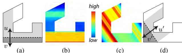
**Figure 5:** Base capacity measured with respect to two base directions, shown in (a) and (d). Only bases that completely cut the shape are considered. Maximal pyramidal parts induced by the bases are colored in light and dark gray. (b) and (c) show color plots of capacity of bases (blue: low; red: high).
