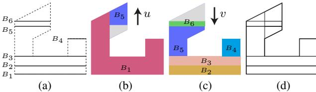
**Figure 7:** Base selection and cell generation. (a) Bases perpendicular to up-vectors  $u$  and  $v$  which received sufficient votes. (b) and (c) show regions of points that voted for the same base (same color with the voted base indicated) with respect to  $u$  and  $v$ . Gray regions contain points who voted for bases that do not have sufficient overall support. (d) Resulting cells when considering only votes collected for the two up-vector directions  $u$  and  $v$ .
