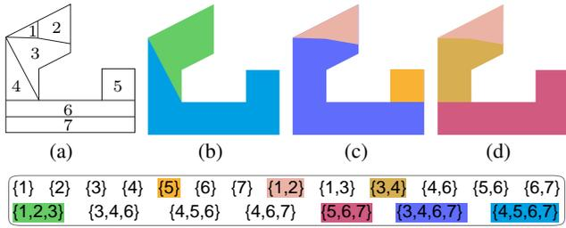
**Figure 12:** Candidate pyramidal parts and pyramidal decompositions via ECP. (a) Input shape and indexed blocks. Bottom shows collection of subsets for ECP, i.e., the set of candidate pyramidal parts, each consisting of a set of blocks. (b) shows the optimal decomposition we found by solving ECP. (c) and (d) show two other decomposition results with more parts. The exact set covers are shown by matching colors in the bottom table.
