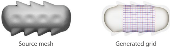
Fig. 7 Cylindrical grid: a mesh with geometric surface details (left), the grid constructed from the base shown in red and blue (right)
