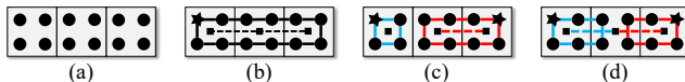
Figure 1: Graph-based CPP and MCPP: Gray squares, black circles, and black stars represent terrain graph vertices, decomposed graph vertices, and initial vertices of robots, respectively; Solid lines and dashed lines represent coverage paths and spanning edges, respectively. (a) Terrain graph with uniform edge weights. (b) The single-robot coverage path generated by STC. (c)(d) Suboptimal and optimal 2-robot coverage paths with makespans 2 and 1.5, respectively.
