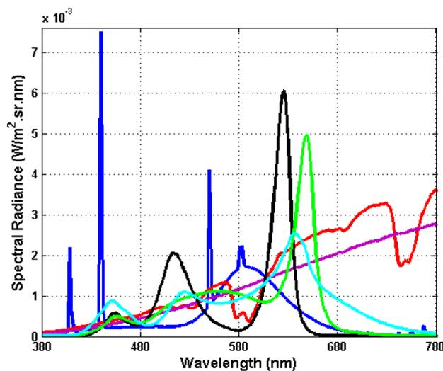
Figure 3: The spectral power distributions of the six light sources (provided by Smet) and used for the comparison of the color rendering measures listed in Table 1. The lights (see text) are F4 (blue curve), FG (green), Nd (red), LC (cyan), H (purple) and RGB (black).
