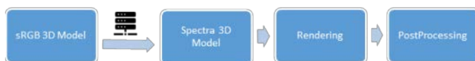
Fig. 6. The process used to generate a full-spectrum image. Begin with an sRGB 3D model, derive a full-spectrum model based on metameric lights and reflectances, use the model to render images wavelength-by-wavelength, and finally combine the renderings into a full-spectrum image.
