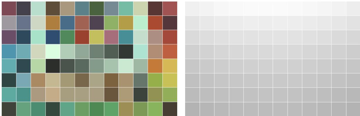
Figure 1. Left: Camera RGB values of the interior patches of the X-Rite Digital ColorChecker SG. Right: The shading arising from irradiance variation on the color checker as measured by removing the color checker and photographing the back wall of the light booth.
