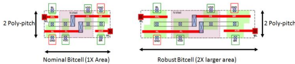
Figure 8: Upsized cell pitch-matched with nominal cell.
