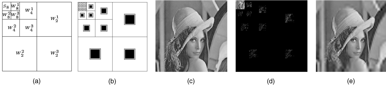
Fig. 1. (a) Discrete wavelet transform. (b) FWT mask \varpi : brick-patterned area—preserved S_8 , deeply shaded area—OFA, lightly shaded area—PPA, and blank area—DPA. (c) Original image \mathcal{I} . (d) FWT \mathcal{F}(\mathcal{I}) . (e) Reconstructed image.
