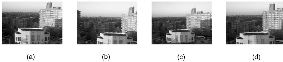
Fig. 5. Effects of pan-tilt-zoom camera movement recovery when there are significant depth differences. (a) and (b) Before and after a pan-tilt movement, (c) and (d) Before and after a zoom movement.
