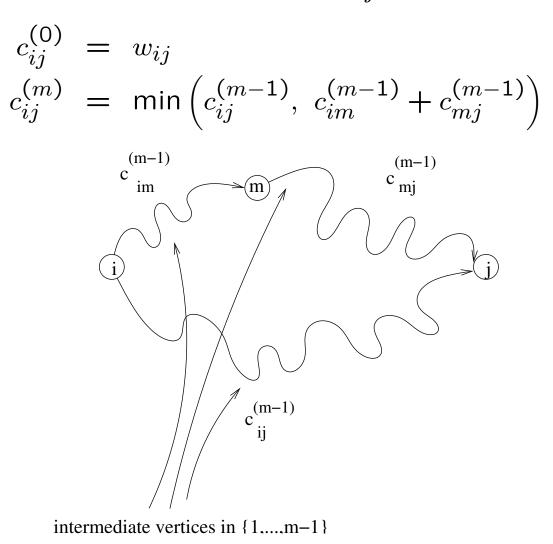
**Difference from previous algorithm:** needn't check *all* possible intermediate vertices. Shortest path simply either includes *m* or doesn't.
