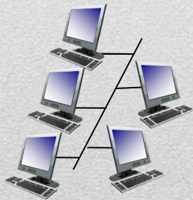
shared wire (e.g., cabled Ethernet)
