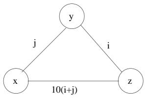
Recall that each node stores its own distance vector and the distance vectors of its neighbors. Assume that the initial phase of the algorithm is over and each node has three correct distance vectors. That is, each node has the information
