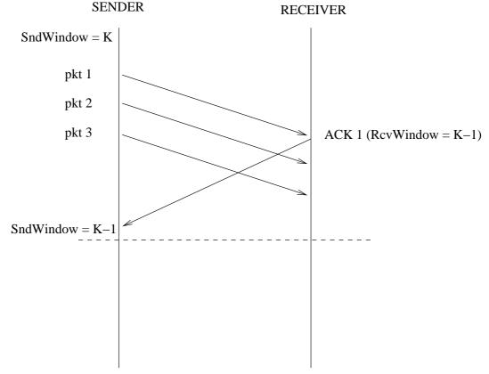
**Solution:** The sender's window has size K - 1 at the dotted line, but the sender has sent 2 packets which have not been acknowledged, so it can send K - 3 packets before it gets another acknowledgement.
