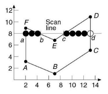
• Could determine span extrema (outermost pixels of a span), using midpoint algorithm, but watch out for extrema outside of polygon (want to fill the interior)
