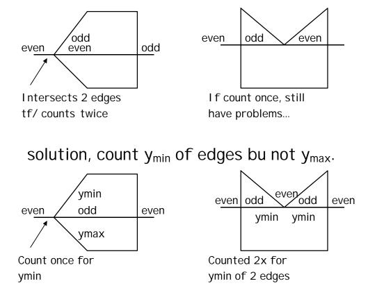
3.4 Horizontal Edges? Bottom edges drawn, top edges not. Since bottom edges will begin with a  $y_{min}$  they will be odd parity.
