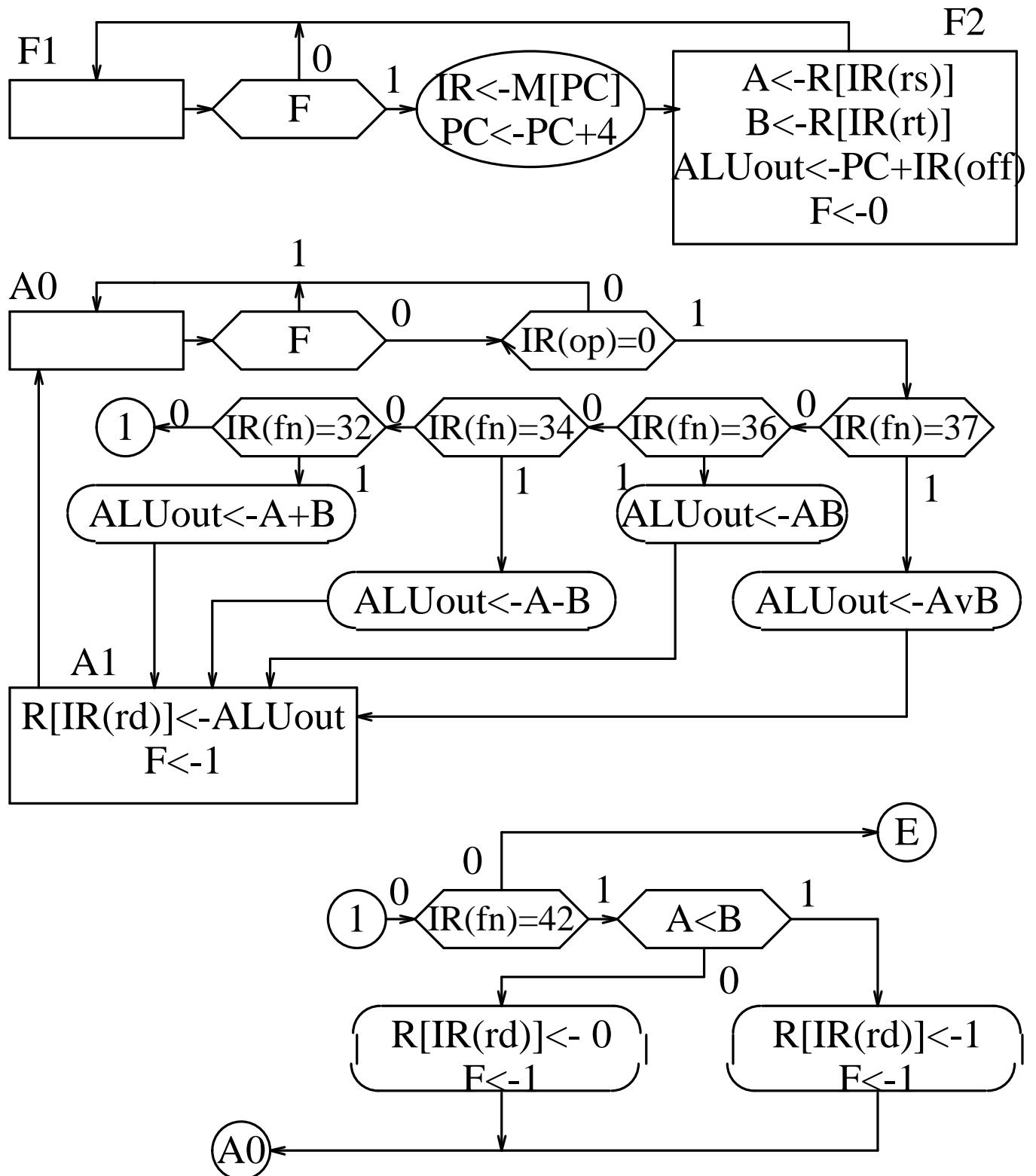
**Figure 3-2:** Fetch and Execute ASM Diagrams Part I
