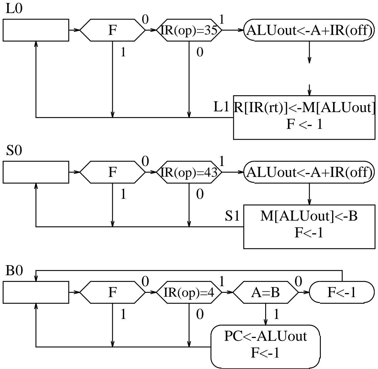
**Figure 3-3:** Execute ASM Diagrams Part II
