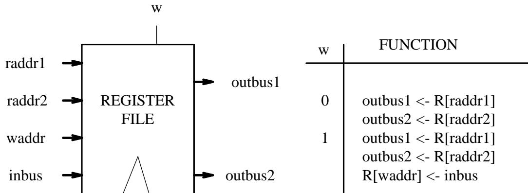
**Figure 2-1:** Behavioral specification of a register file
