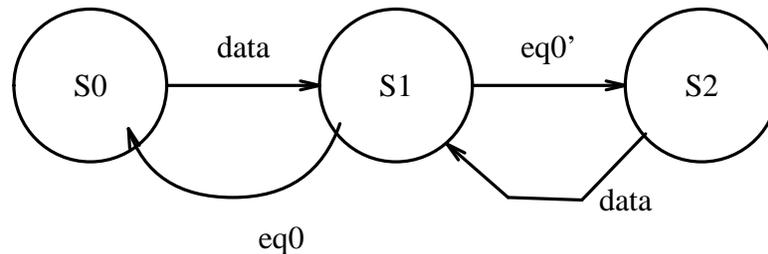
**Figure 6-1:** State Diagram for the Sequencer of the SUM Circuit
