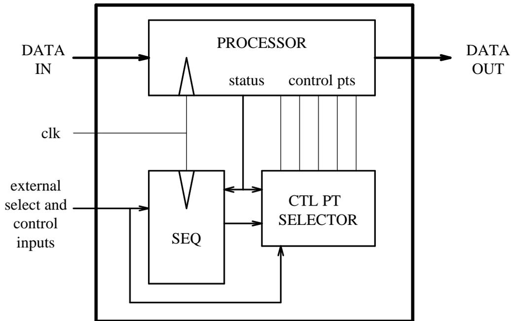
**Figure 4-1:** Typical System Architecture from ASM Design
