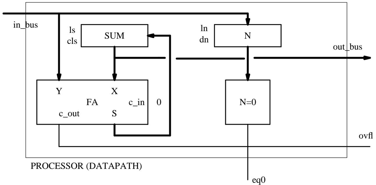
**Figure 5-1:** Processing Component of the SUM Circuit
