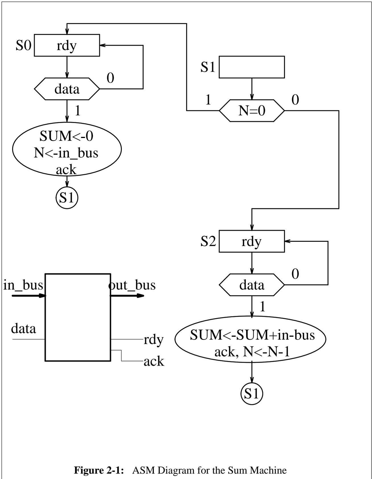
**Figure 2-1:** ASM Diagram for the Sum Machine
