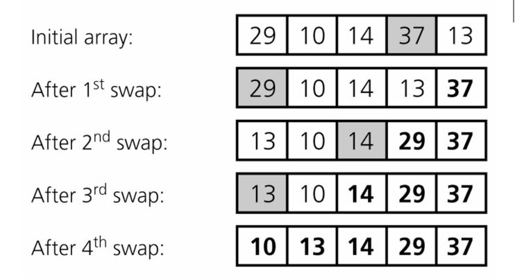
A selection sort of an array of five integers (using the algorithm in the textbook, in which the first part of array is unsorted and the second (bold) is sorted. Instead of the smallest element we have to look for the biggest element.
