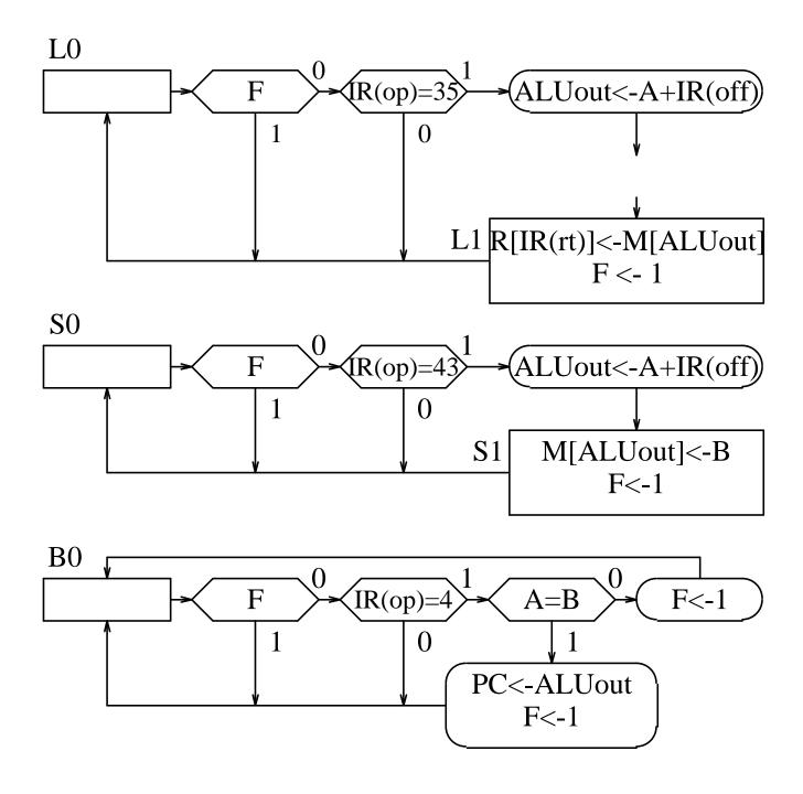
Figure 3-3: Execute ASM Diagrams Part II
