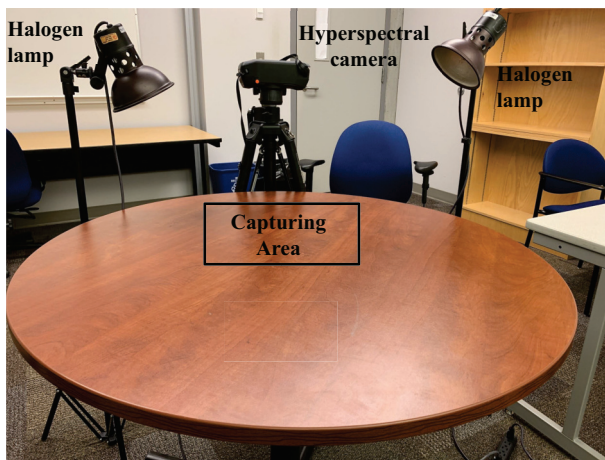
Figure 7: The experimental setup used to capture hyperspectral images of hands and arms of human subjects.
